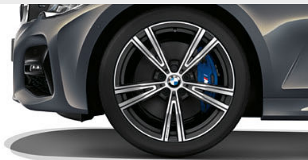
□ 19" BMW Individual light alloy wheels Double-spoke style 793 in Bicolour Orbit Grey with mixed tyres and runflat tyres, burnished, front 8J x 19 with 225/40 R19 tyres, rear 8.5J x 19 with 255/35 R19 tyres.
