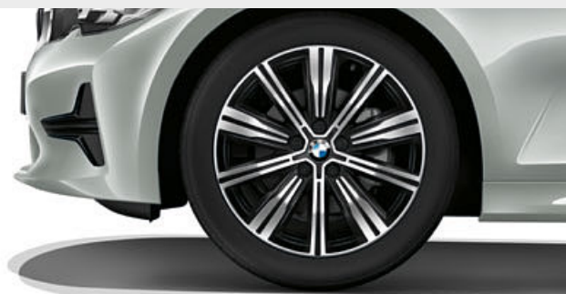
□ 18" light alloy wheels Double-spoke style 782 Bicolour Jet Black, gloss-lathed, wheel size 7.5J x 18 with 225/45 R18 tyres.
