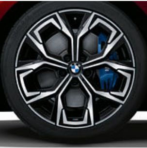
□ 19" M aerodynamic wheels 860 M Bicolour Black Grey with mixed tyres, gloss-lathed, wheel size front 8.5J x 19 with 245/40 R19 tyres, wheel size rear 9J x 19 with 255/40 R19 tyres. 2
