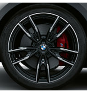
19" M light alloy wheels Double-spoke style 792 M Bicolour Jet Black with mixed tyres and runflat tyres, gloss-lathed, front 8J x 19 with 225/40 R19 tyres, rear 8.5J x 19 with 255/35 R19 tyres. 4
