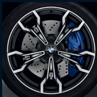
□ 21" M light alloy wheels V-spoke style 765 M Bicolour Jet Black with mixed tyres, gloss-lathed, front wheel size 9.5J x 21 with 255/40 ZR21 tyres, rear wheel size 10J x 21 with 265/40 ZR21 tyres.
