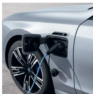
The fast charging cable (mode 3) allows you to charge the high-voltage battery at public charging stations – 3-phase and with a charging capacity of up to 7,4kW.
